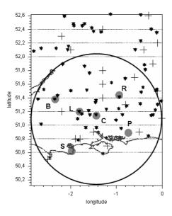
Figure 6.1: Locations of some of the instrumentation deployed in southern Britain during the CSIP campaign. The stars represent the positions of the AWS and SYNOP stations. The crosses indicate the positions of the GPS sites. The circles represent the positions of the six radiosonde stations Bath (B), Swanage (S), Larkhill (L), Chilbolton (C), Reading (R), and Preston Farm (P). The ring centered on Chilbolton indicates the 100 km range of the Chilbolton radar.
