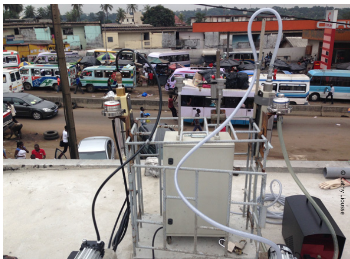
Three aerosol impactors are running in parallel at each WP2 site: here at the traffic site of Adjamé at Abidjan in Ivory Coast.
