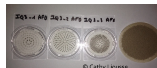
Example of collected filters with aerosol impactors at the domestic fire site of Yopougou (Abidjan in Ivory Coast): IQ3-1 filter (on the left) include particles larger than PM 2.5 , IQ3-2, (PM 1 - PM 2.5 ), IQ3-3, (PM 0.2 -PM 1 ) and the back up filter (on the right) with particles smaller than PM 0.2 .
