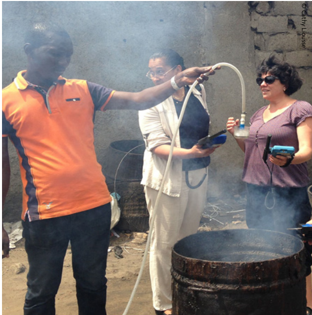
Emission factor measurements above a domestic rubberwood fire at Yopougon in Ivory Coast with filters, CO/CO 2 and VOC sampling.
