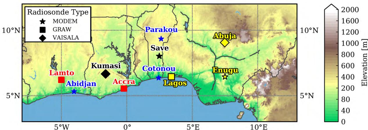
*DACCIWA Radiosonde network and deployed sonde types. Blue: Operational or re-activated AMMA stations with enhanced sounding frequency; Black: DACCIWA super-sites; Red: DACCIWA stations operated by KIT, GMet, and UFHB; Yellow: Operational ASECNA and NWS stations outside the DACCIWA network*
