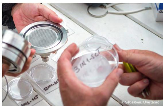
Filters with aerosol impactors
