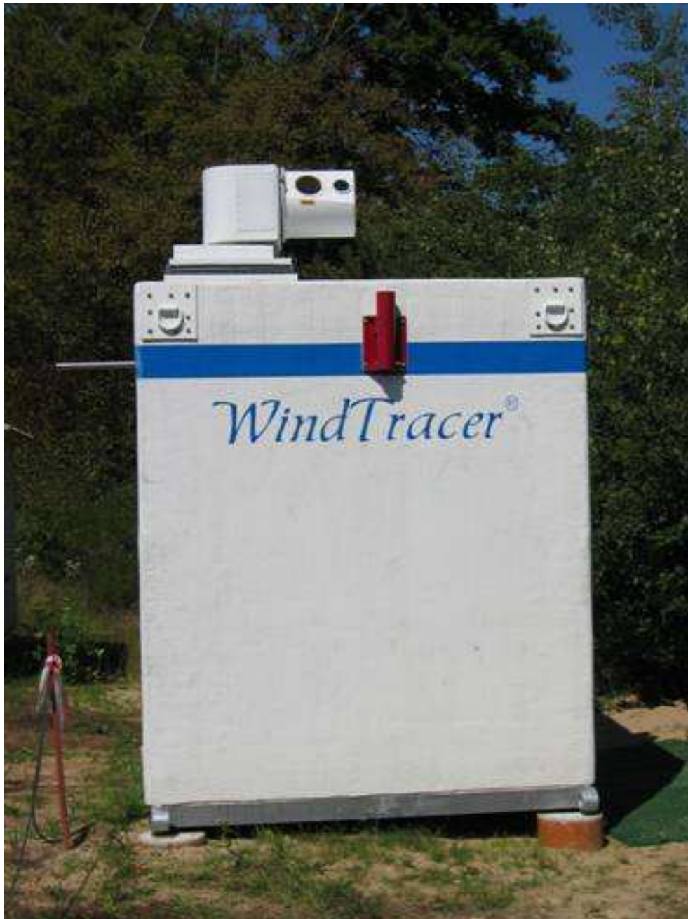
Figure 6: The CLR Photonics Wind Tracer a coherent Doppler lidar, at its site at the FZK.
