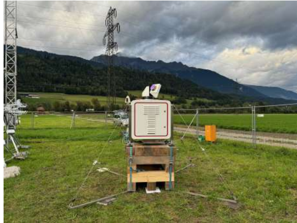
Figure 3.4.: Leosphere/Vaisala Windcube WLS200s at the observation site Kolsass. Photo: Andreas Wieser.
