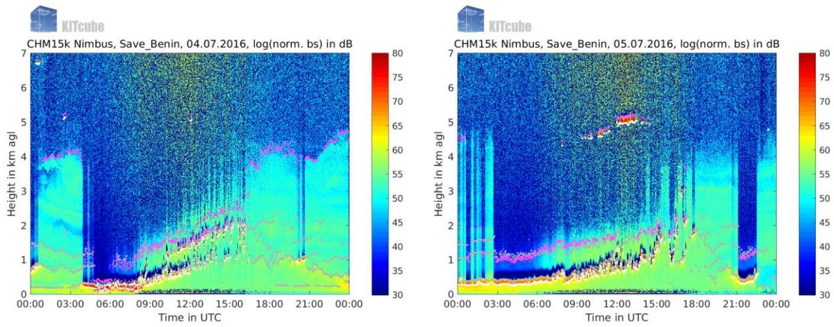
Figure 17: Ceilometer backscatter (colour-coded) at Savè during IOP 7. White dots indicate cloud base.
