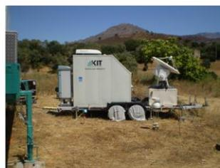
Fig.1: MIRA36-S cloud radar (Metek Comp., Elmshorn, Germany) Fig.2: MIRA36-S cloud radar, in field campaign.
