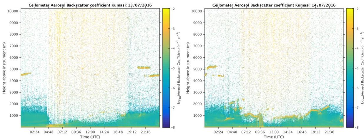
Figure 24: Ceilometer backscatter (colour-coded) at Kumasi during IOP 10.
