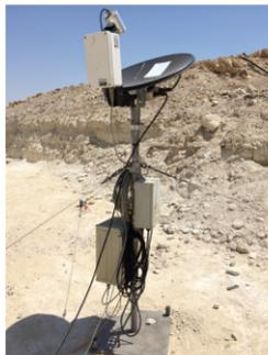
Fig. 1: The K-band Doppler Radar FCMW
