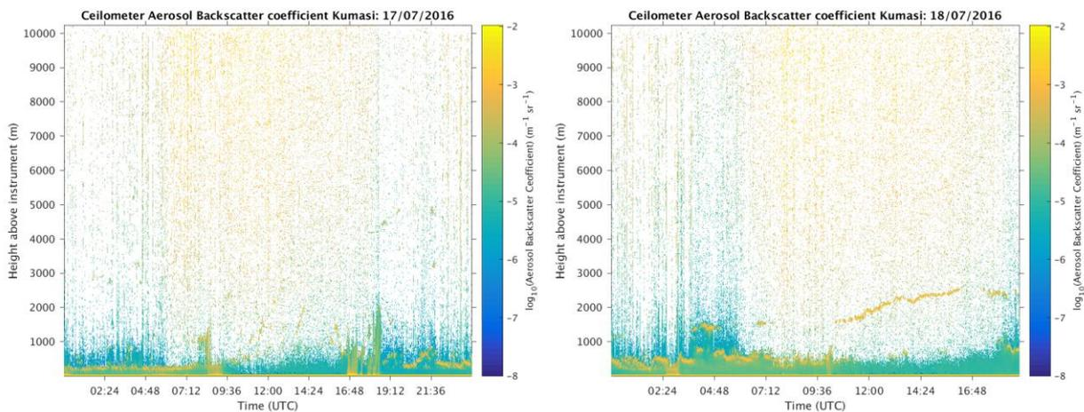
Figure 26: Ceilometer backscatter (colour-coded) at Kumasi during IOP 11.
