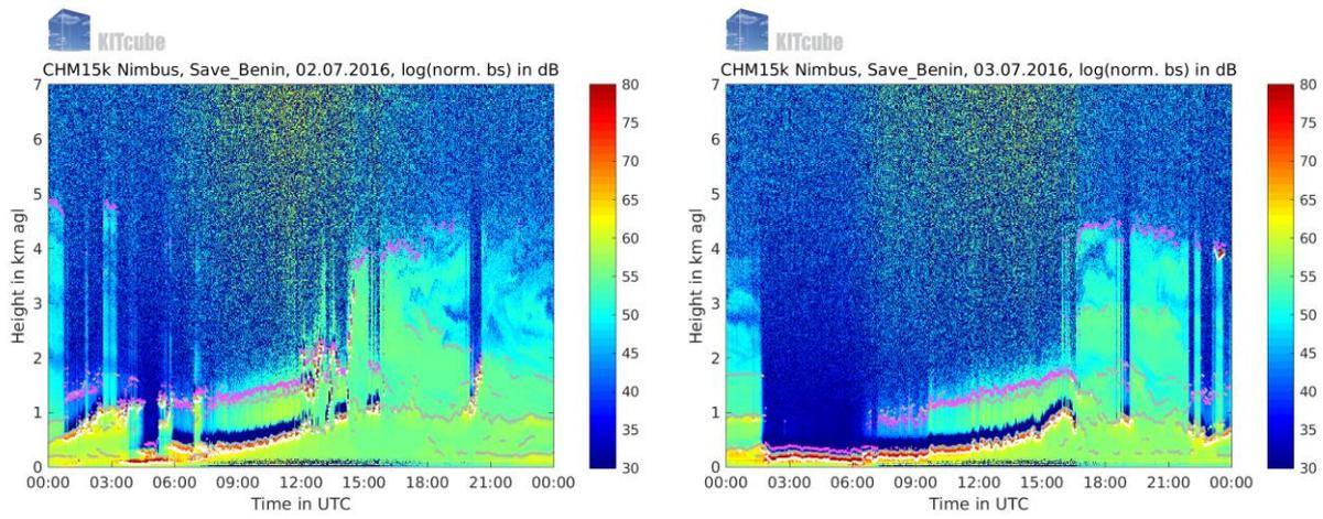
Figure 15: Ceilometer backscatter (colour-coded) at Savè during IOP 6. White dots indicate cloud base.
