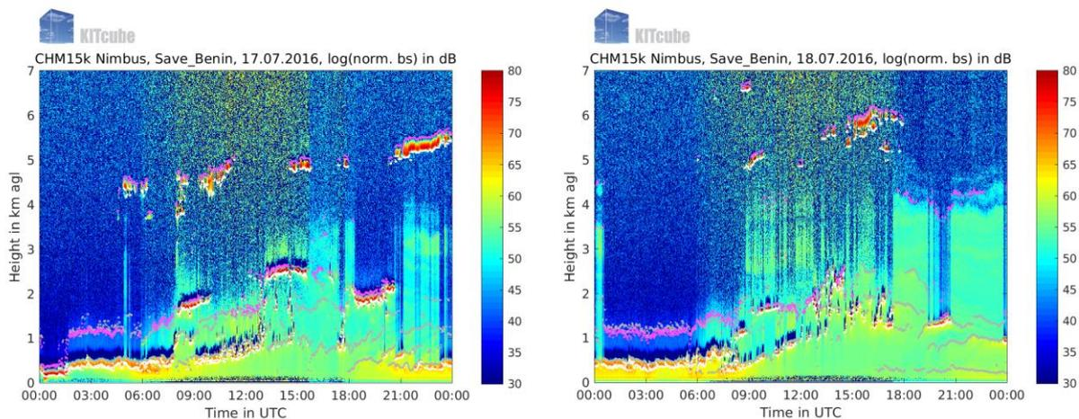
Figure 25: Ceilometer backscatter (colour-coded) at Savè during IOP 11. White dots indicate cloud base.
