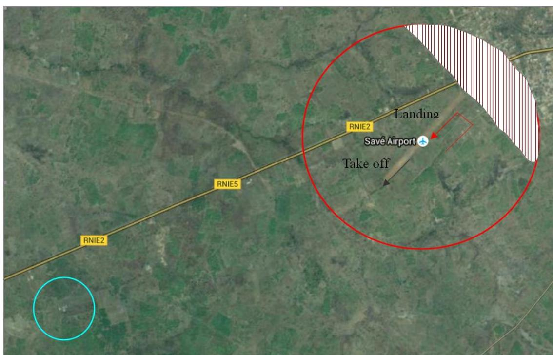
*Fig. 3: Overview of airfield sites at Savé. The red circle stands for the 1 km radius zone for the RPAS Aladina operation. The white area is excluded from the ALADINA operation because of the city. The blue circle stands for the zone for the RPAS OVLITA operation.*
