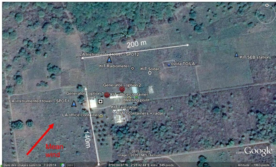
Fig. 7: Instrumentation map at Gobe site.
