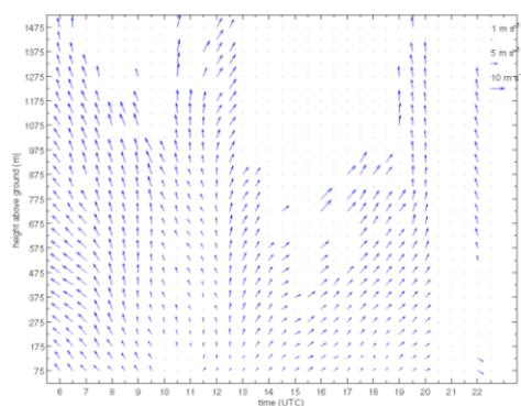
Fig. 4: Using well-known algorithms (VAD), the measured wind information during a PPI scan can be used to determine vertical profiles of horizontal windspeed and direction.
