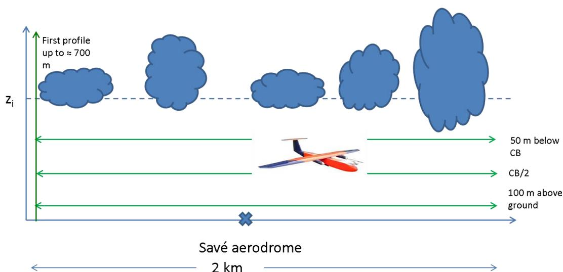
Fig. 17: Flight pattern for RPAS Aladina for breaking stratus and convective clouds.
