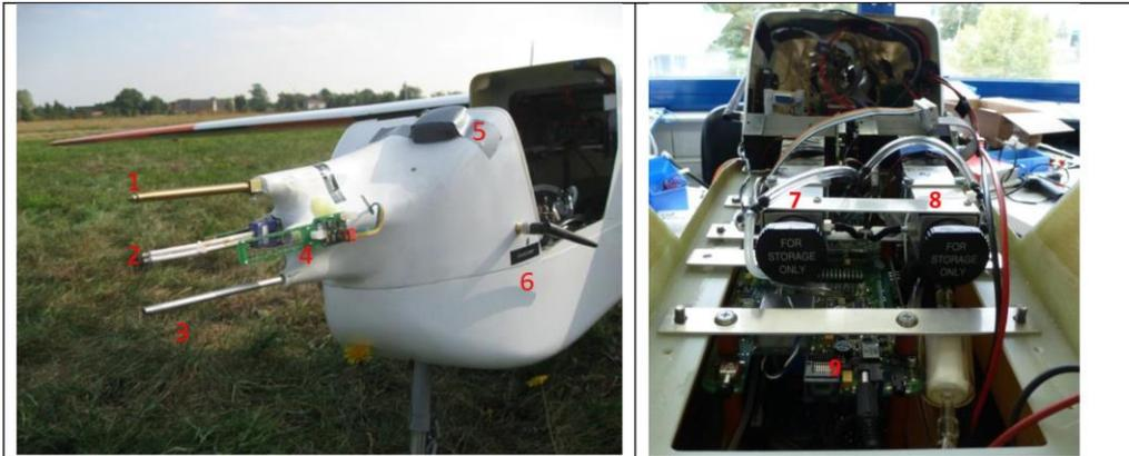
ALADINA payload: 1 five-hole probe, 2 temperature and humidity sensor, 3 aerosol inlet, 4 temperature sensor, 5 GPS antenna, 6 telemetry antenna b) 7, 8, 9 aerosol instruments
