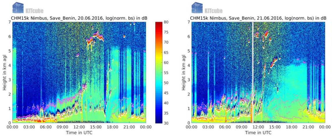
Figure 7: Ceilometer backscatter (colour-coded) at Savè during IOP 2. White dots indicate cloud base.
