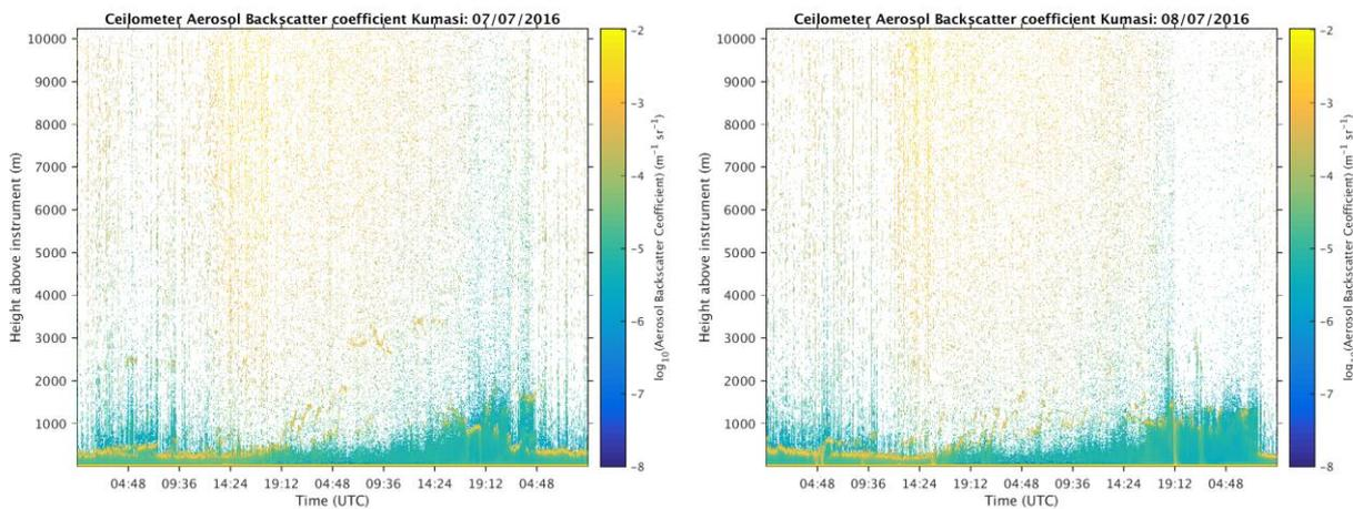
Figure 20: Ceilometer backscatter (colour-coded) at Kumasi during IOP 8.
