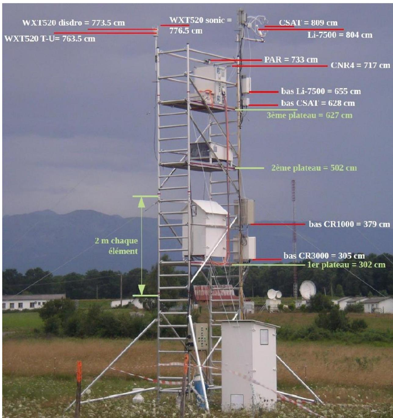
Figure: Surface station for energy balance and biogenic fluxes.
