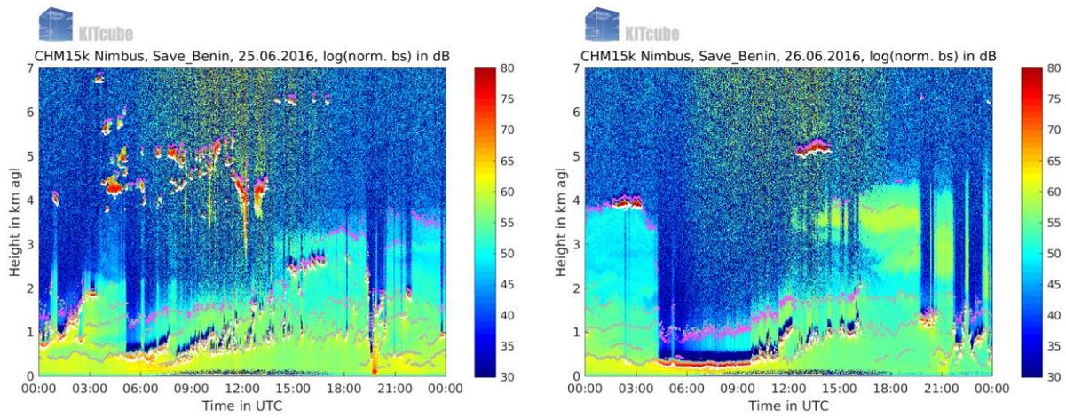
Figure 9: Ceilometer backscatter (colour-coded) at Savè during IOP 3. White dots indicate cloud base.
