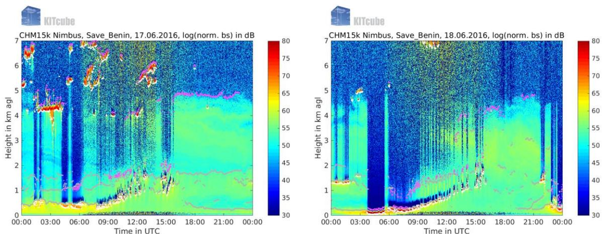
Figure 5: Ceilometer backscatter (colour-coded) at Savè during IOP 1. White dots indicate cloud base.
