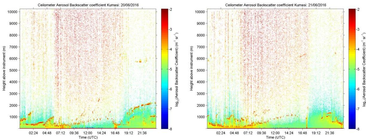
Figure 8: Ceilometer backscatter (colour-coded) at Kumasi during IOP 2.
