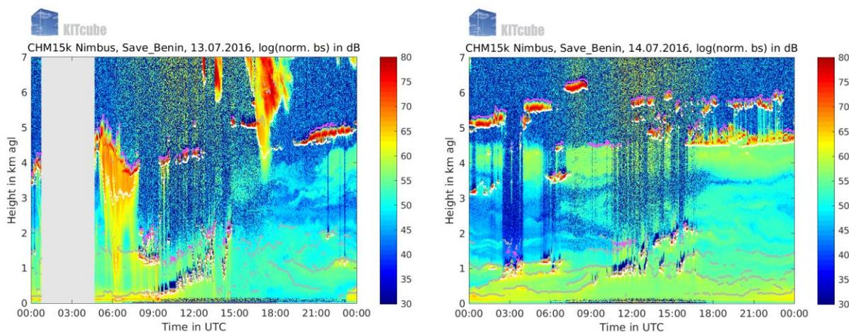
Figure 23: Ceilometer backscatter (colour-coded) at Savè during IOP 10. White dots indicate cloud base.
