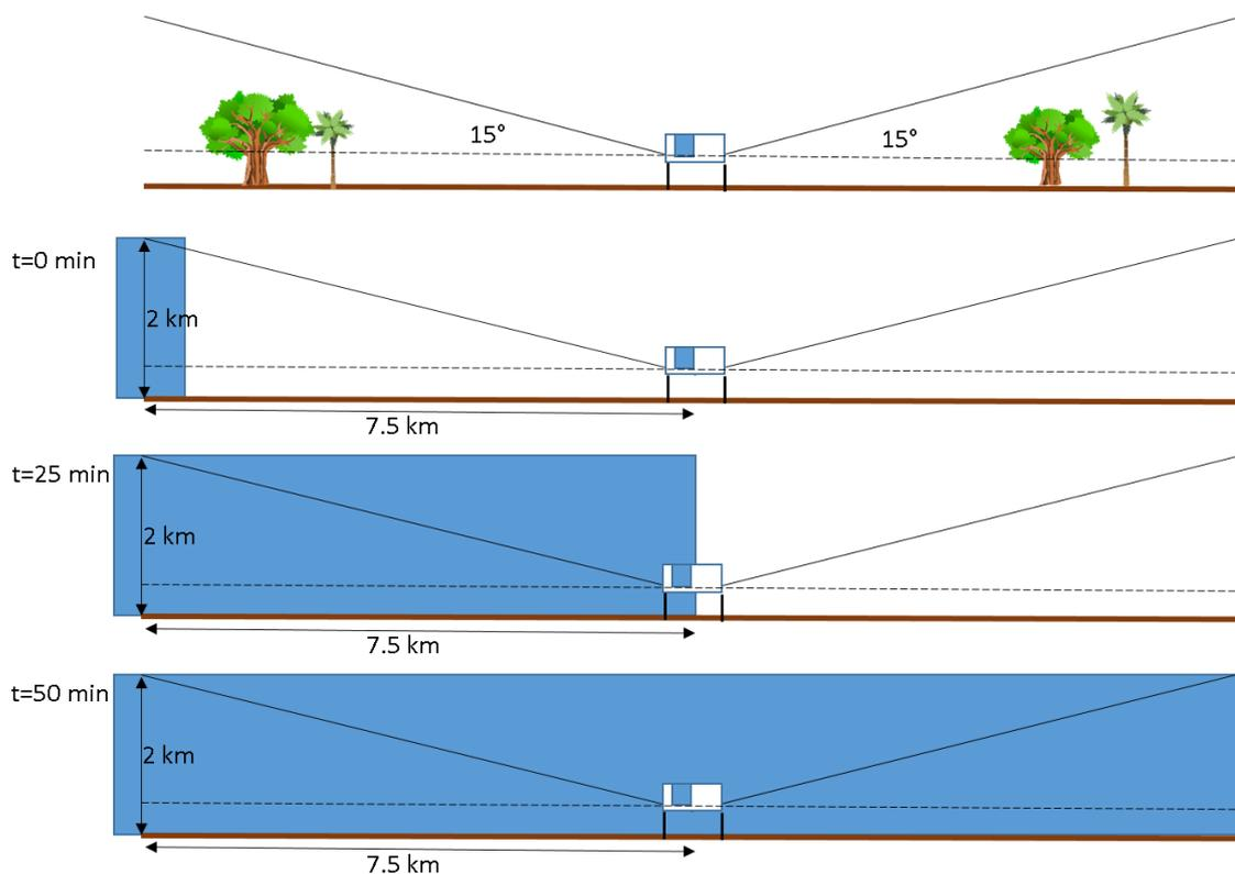
Fig. 10: Schematic diagram to illustrate the PPI of the microwave radiometer at Savé
