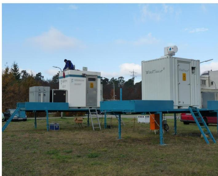
Fig. 2: "WindTracer" systems delivered in 2004 (rear) and 2009 (front). Both systems are installed on loading bridges, allowing easy transportation.
