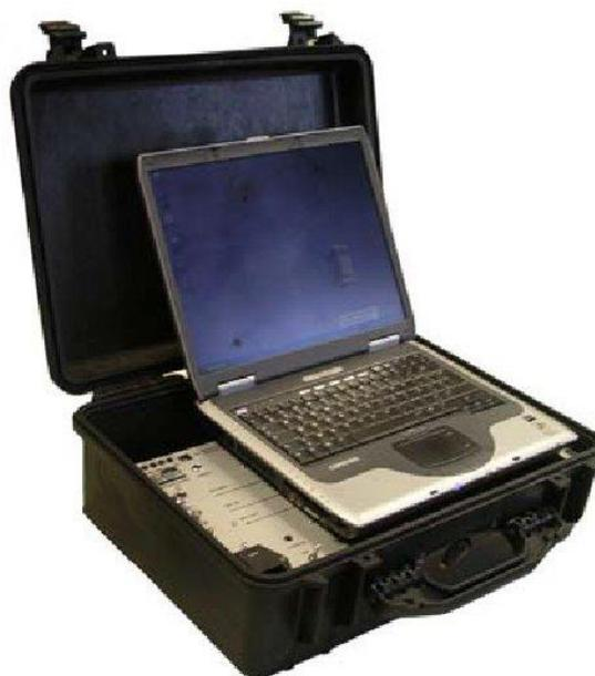
*Figure: MODEM Radio sounding System*
