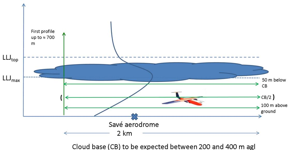
Fig. 16: Flight pattern for RPAS Aladina for nocturnal stratus.
