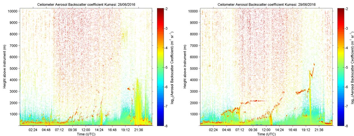
Figure 12: Ceilometer backscatter (colour-coded) at Kumasi during IOP 4.
