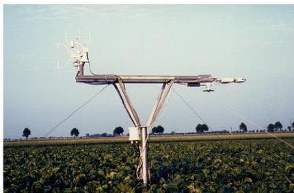
Fig.1: Energy balance station to register the energy conversion of the ground
