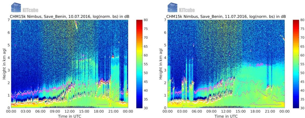
Figure 21: Ceilometer backscatter (colour-coded) at Savè during IOP 9. White dots indicate cloud base.
