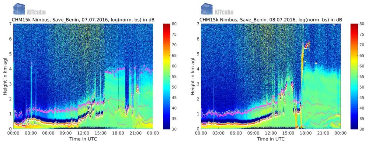
Figure 19: Ceilometer backscatter (colour-coded) at Savè during IOP 8. White dots indicate cloud base.
