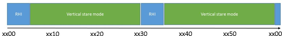
Fig. 13: Time line of scans performed with the wind lidar *WindTracer* and the cloud radar at Savé.
