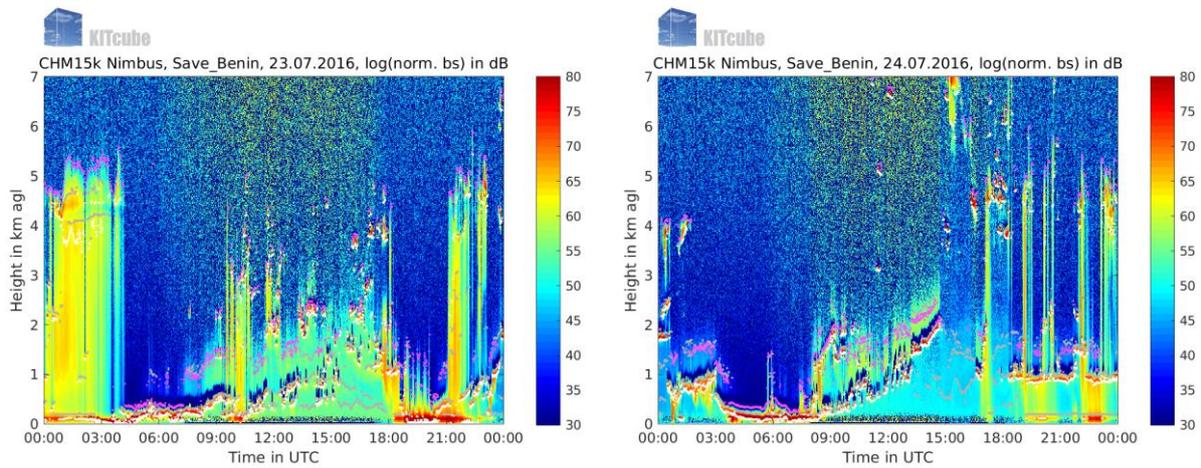
Figure 29: Ceilometer backscatter (colour-coded) at Savè during IOP 13. White dots indicate cloud base.
