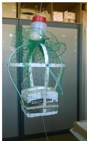
*Figure: On the left the sonde with the ascent (white) and descent (red) balloons. On the right, the sonde MODEM M10 with its protection.*
