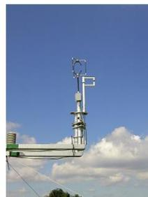
Fig.2: Ultrasonic anemometer and Lyman-Alpha hygrometer of a energy balance station
