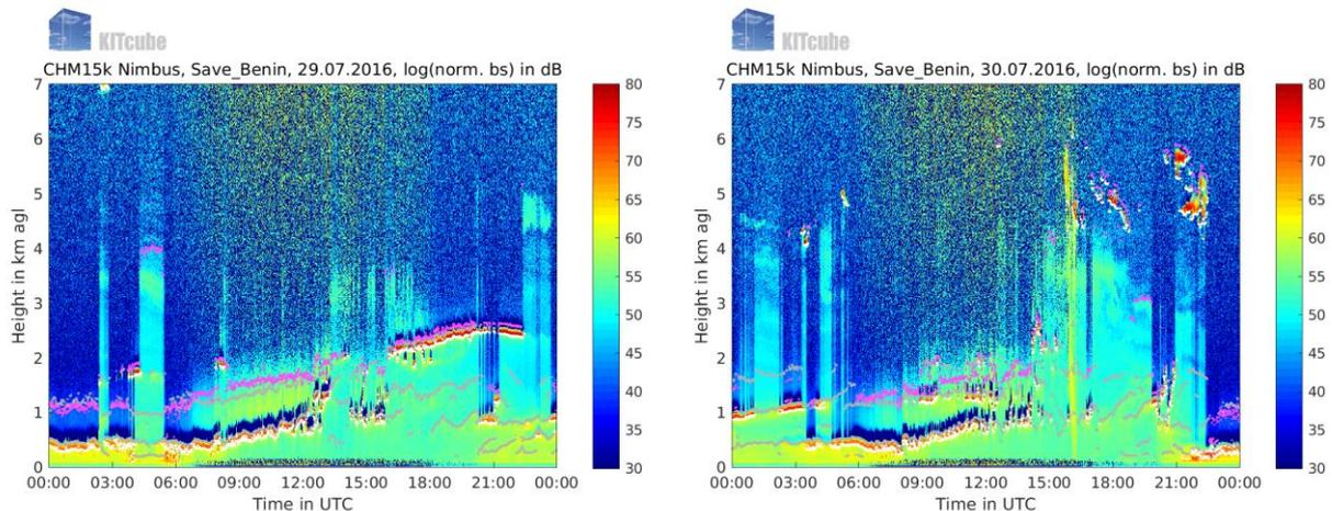
Figure 33: Ceilometer backscatter (colour-coded) at Savè during IOP 15. White dots indicate cloud base.
