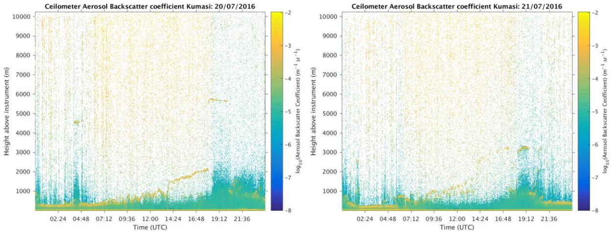
Figure 28: Ceilometer backscatter (colour-coded) at Kumasi during IOP 12.
