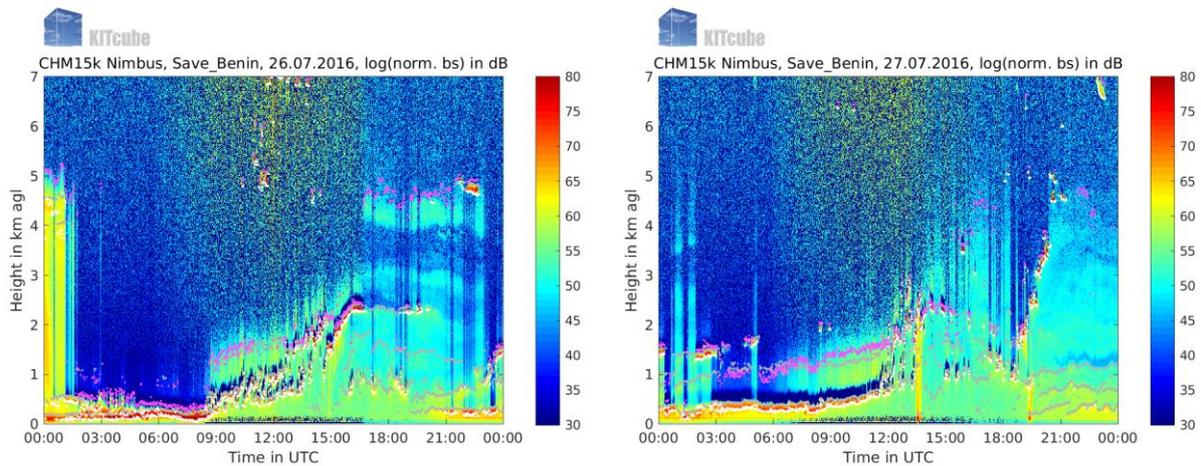
Figure 31: Ceilometer backscatter (colour-coded) at Savè during IOP 14. White dots indicate cloud base.
