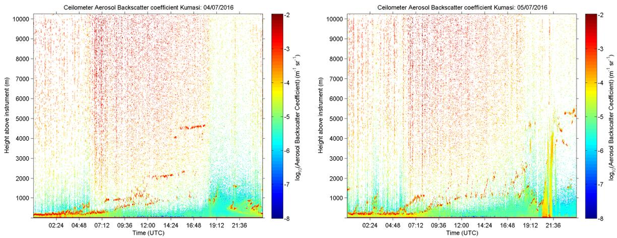
Figure 18: Ceilometer backscatter (colour-coded) at Kumasi during IOP 7.
