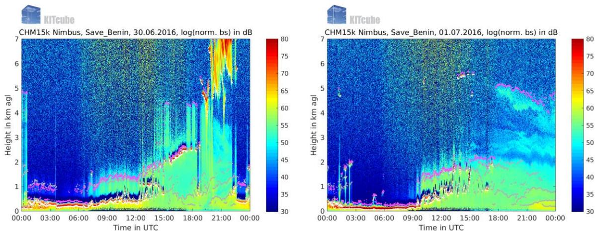
Figure 13: Ceilometer backscatter (colour-coded) at Savè during IOP 5. White dots indicate cloud base.
