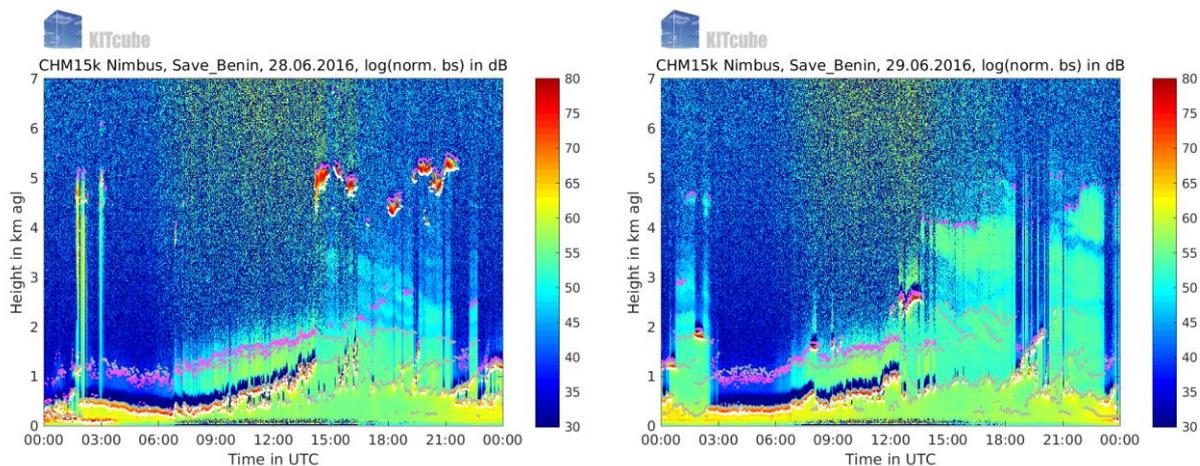
Figure 11: Ceilometer backscatter (colour-coded) at Savè during IOP 4. White dots indicate cloud base.
