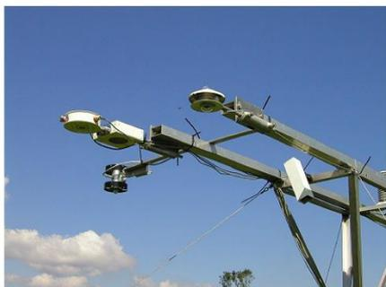
Fig. 3: Radiance measuring instruments on an energy balance station
