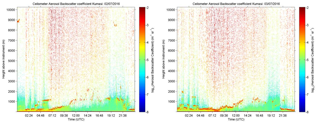
Figure 16: Ceilometer backscatter (colour-coded) at Kumasi during IOP 6.
