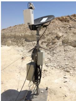
Fig. 1: The K-band Doppler Radar FCMW
