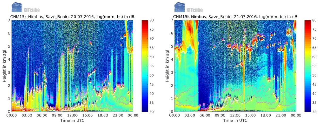
Figure 27: Ceilometer backscatter (colour-coded) at Savè during IOP 12. White dots indicate cloud base.
