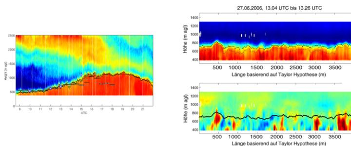
Fig. 5: High-resolution measurements of the signal-to-noise ratio and the vertical wind speed provide the ability to detect variations in the boundary layer height at different temporal scales: small-scale events in the order of less than 10 m, which can be associated with entrainment processes but also complete diurnal variations of the atmospheric boundary layer can be measured. Here are two examples of the CSIP field campaign, 2005.
