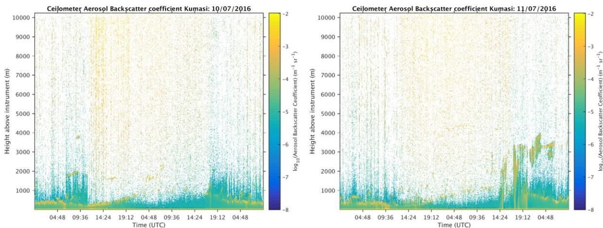
Figure 22: Ceilometer backscatter (colour-coded) at Kumasi during IOP 9.
