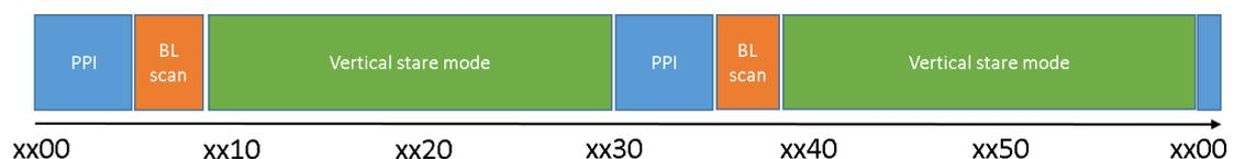
Fig. 11: Time line of the scan strategy performed with the microwave radiometer at Savé.
