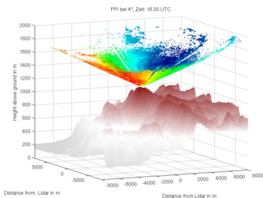
Fig. 3: So-called Plan-Position-Indicator scans (PPI) measure along conical cross sections. Here an example measured during the COPS field campaign (2007) is shown. This method gives an impression of the 3D wind field, bearing in mind that the wind can always be determined only in the beam direction
