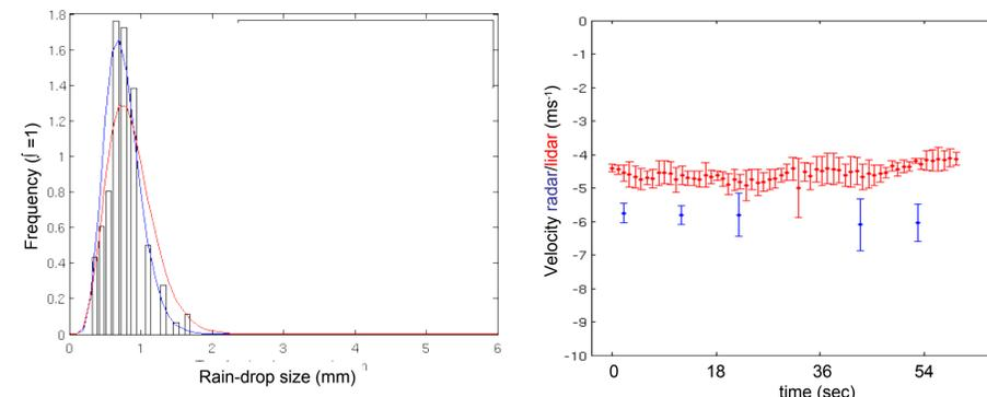
Fig. 3 (left): Rain-drop size-distribution from Disdrometer (bars), estimated distribution from moments of the Disdrometer measurement (blue) and from estimation using the radar and lidar velocities (red). Fig. 3 (right): vertical velocities associated to the spectra.
