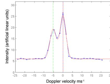
Fig. 2: Double peaks in the lidar Doppler spectra during rain: measured spectra (blue), Gauss fit (red) and two maxima indicated by vertical green and red line. One peak has always a velocity lower than zero, the other approx. zero.
