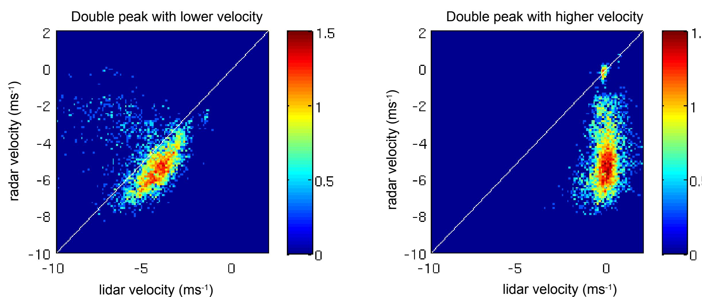
Fig. 1: Comparison of approx. 10.000 simultaneously measured vertical velocities. The lidar is able to detect 2 peaks (Fig. 2) in the Doppler spectra, a rain peak (left) and an air peak (right); the colour scale is in logarithmic units.
