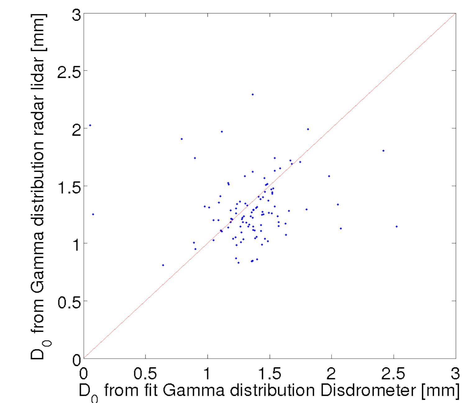
Fig. 4: Comparison between  $D_0 = \mu + \frac{4}{\lambda}$  from Disdrometer and estimated from the radar/lidar combination.
