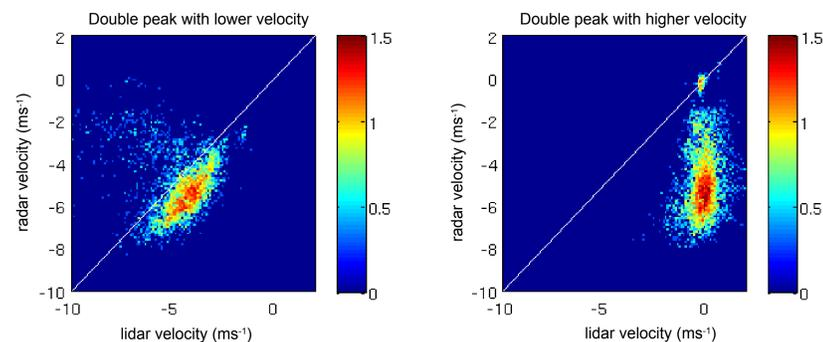
Fig. 1: Comparison of approx. 10,000 simultaneously measured vertical velocities. The lidar is able to detect 2 peaks (Fig. 2) in the Doppler spectra, a rain peak (left) and an air peak (right); the colour scale is in logarithmic units.
