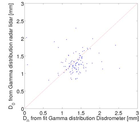
Fig. 4: Comparison between  $D_0 = \mu + 4/\lambda$  from Disdrometer and estimated from the radar lidar combination.
