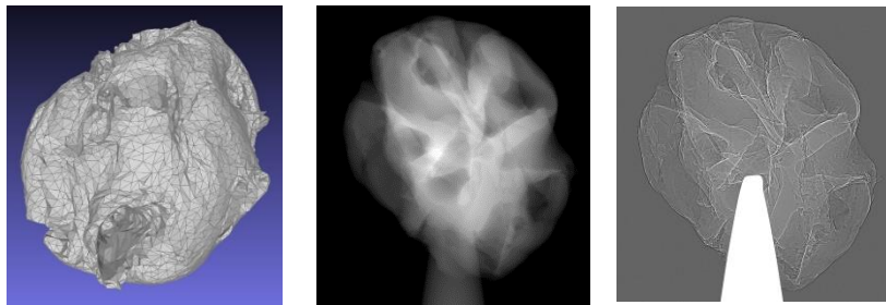
Figure: (left to right) a 3D mesh visualization, its projected thickness and X-ray simulation.
