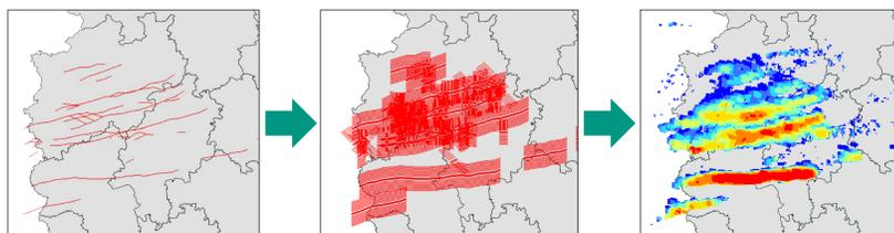
Fig. 4: Thunderstorm tracks on one day (middle) by TRACE3D (Handwerker, 2002), duplication of shifting vectors (middle) and interpolation of the hail criterion HC parallel to the tracks (right).
