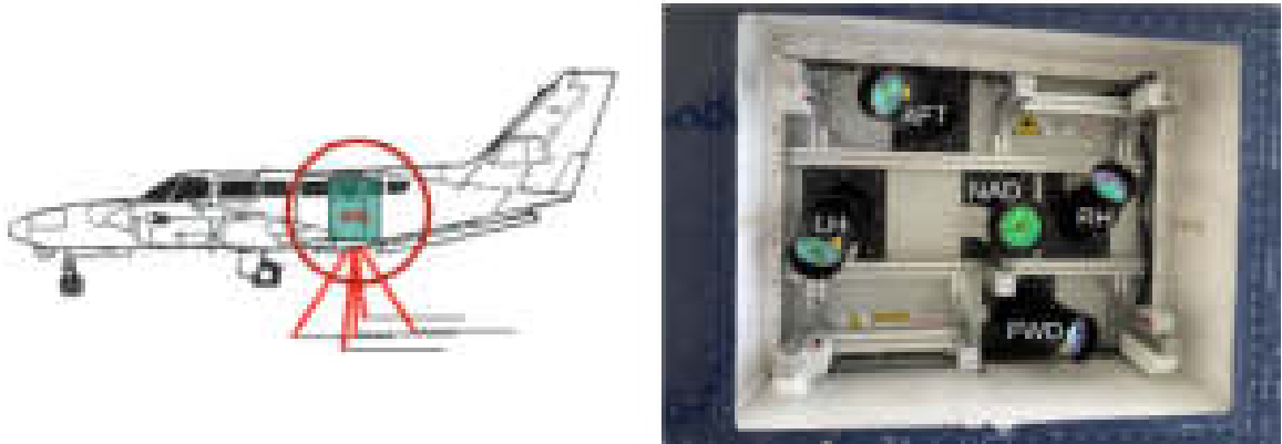
Figure 3.6.: Left: Sketch of the Cessna 406 research aircraft of the Technische Universität Braunschweig with the airborne Doppler lidar (ADL) system AIRflows on board. Right: Photo of the five Doppler lidars of the AIRflows system pointing in fixed directions, photographed from below the aircraft. Courtesy of Dr. Philipp Gasch, combined by the author.
