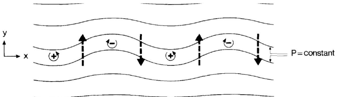
Figure 3.3: Figure 17 from Hoskins et al. (1985): Schematic IPV map of a x-periodic Rossby wave train in an initial northward IPV gradient in a westerly base flow. The contours of IPV are deflected, leading to positive (+) and negative (-) IPV anomalies. The dashed arrows show the induced wind field, leading to a westward propagation of the Rossby wave train with respect to the base flow.
