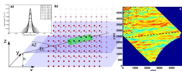
Fig. 2: a) Relative weights of radial velocity around lidar range gate center in velocity estimation b) Sketch of lidar simulator c)  $u'$  from DD-lidar retrieval, the dashed line indicates the direction of wavelet analysis.
