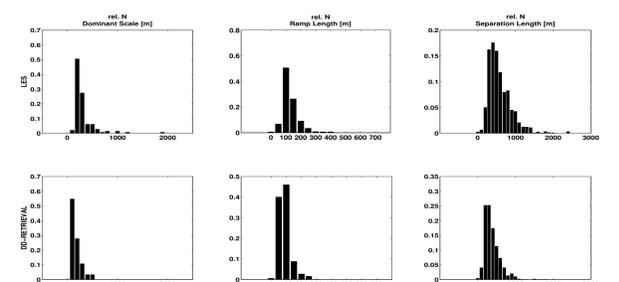
Fig. 7: Accumulated wavelet analysis results in spanwise direction: Relative frequency of dominant scales, ramp lengths and separation lengths.
