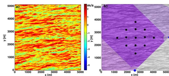
Fig. 1: a) The turbulent windfield component in streamwise direction,  $u'$ , from LES data at 10 m height. b) Virtual lidar positions in LES area (blue dots) and virtual tower positions (black dots). The lidar scan areas are shaded, the dark shade is the lidar beam overlap region.
