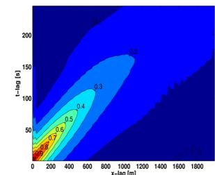
Fig. 6: Correlation coefficient of streamwise wind field LES data in 10 m height with x-lag in streamwise direction and t-lag along the time axis
