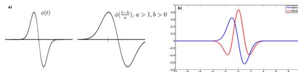
Fig. 3: a) Stretching and shifting of wavelet function. b) 'Wave' and 'Mexican Hat' wavelets
